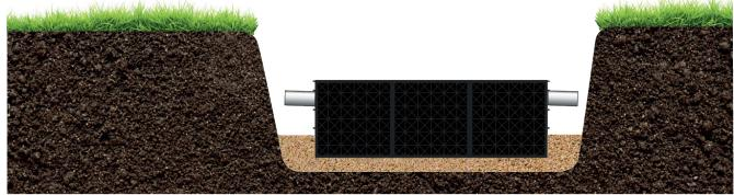
**3.** Connect up the pipework (and if necessary a sand filter). Continue filling with drainage sand up to 10 cm above the infiltration crates. If the area above is to be planted, place a sheet of plastic over the infiltration system and cover with earth.
